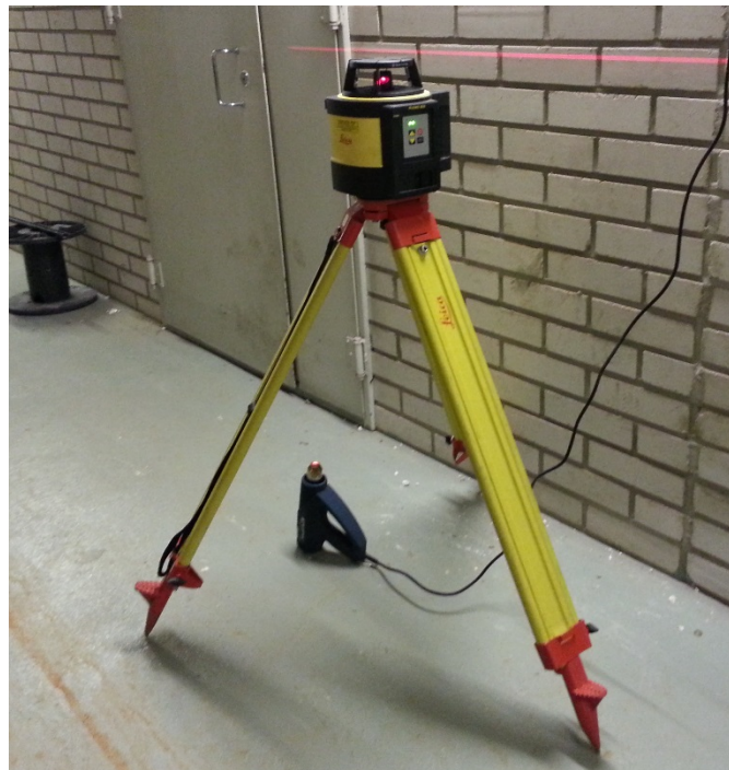
Fig. 1. Creating artificial air turbulence using a hot air blower.
