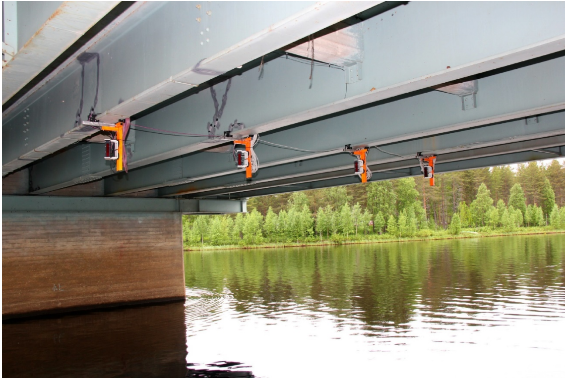
Four DMM sensors measuring deflection of main girders.
