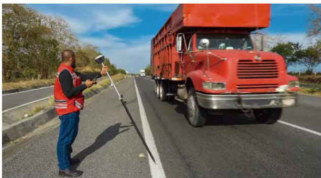
Figure 5.1 Tilt survey- on the high way
